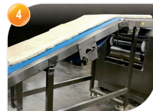
4 面带松弛输送 (1次) Dough sheet resting (First)
