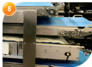
8 滑轨式三层输送设计 (延长松弛时间) Slide rail type three-level conveyor design (Extend resting time)
