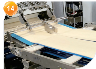
14 第三道厚度成形杆压 Finally thickness kneading process
