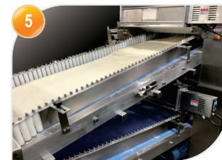
5 面带压面 (PLC伺服传动控制) Dough kneading/sheeting process (Servo transmission)
