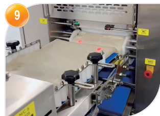
9 入面输送→杆压 Deliver dough sheet, ready for kneading
