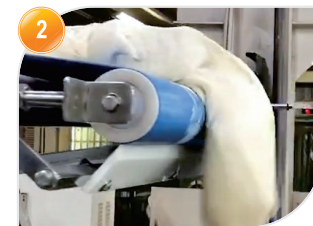
2 面带爬升设计 Dough sheet climbing design
