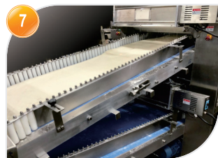
7 面带压面 (PLC伺服传动控制) Dough kneading/sheeting process (Servo transmission)
