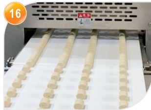
16 伺服切断传动 Cutting transmission by servo control system
