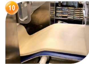
10 杆压 Kneading / Sheeting process
