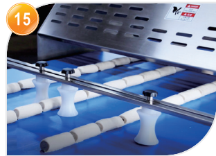
15 分流4条产线 (产能4倍) Separate 3 lines for forming production (Capacity triple)
