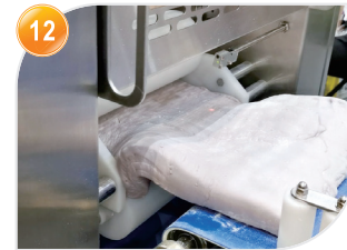
12 第一道轮入面杆压 Main first kneading process
